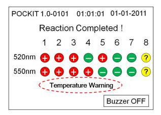
Caution: Fluctuation of ambient temperature should not be more than 5°C during the reaction.
