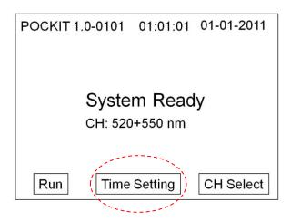
2) Touch the numbers that needs to be changed on the screen. Press "Up" and "Down" buttons to select the desired number. Press "OK" to confirm and return to the "System Ready" screen. Press "Cancel" to quit and leave the "Time Setting" screen.
