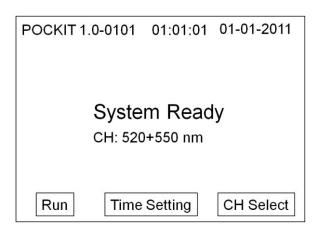
3) Before the reaction starts, to change the detection wavelength, press "CH Select" and choose again.
